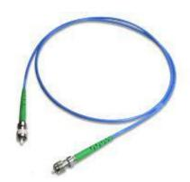
These polarization-maintaining fiber optic patch cables are terminated on both ends with high-quality, narrow key, ceramic FC/PC connectors, featuring high-quality polish with a typical return loss of 50 dB. Each cable is individually tested to ensure the specified extinction ratio and insertion loss at fiber-to-fiber junctions. Each patch cable includes two protective caps that shield the ferrule ends from dust and other hazards. Each cable comes with a mating connector adaptor for ease of use.
